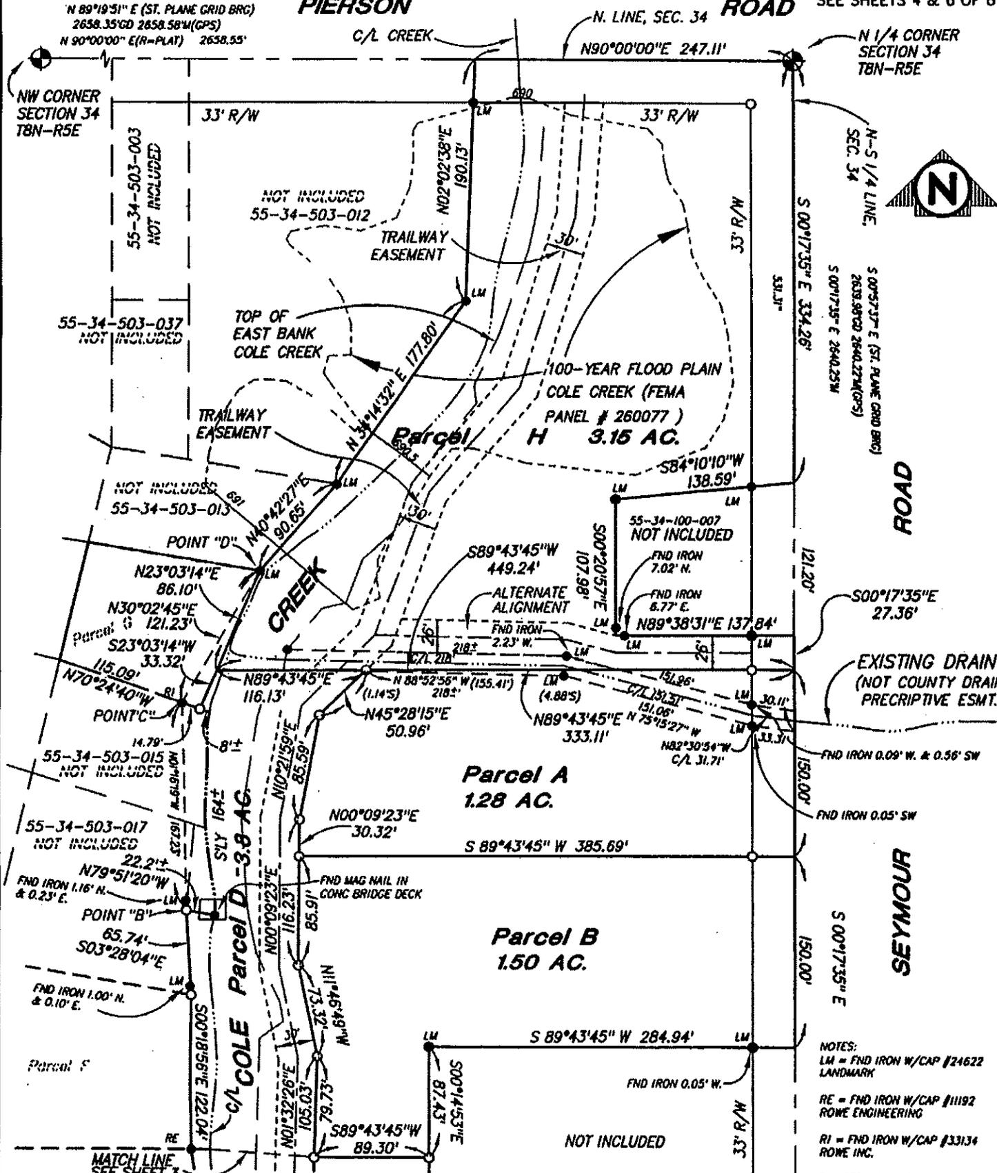
BEARINGS ARE REFERENCED TO N. LINE OF SECTION 34, PER COLE CREEK NO. 4, L. 53, P. 5-6, G.C.R.
